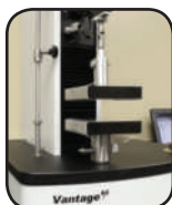
Film Blocking Fixture ASTM D3354
