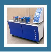
The RK-21 is an automatic sheet former used for the production of laboratory hand sheets in accordance to the Rapid Köthen method for measurement of the physical and/or optical properties of pulps.
