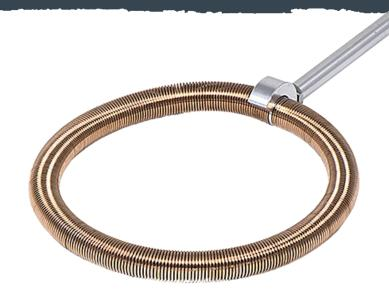
The Rolling Spring is for the testing of coatings on the external diameter of pipes.
