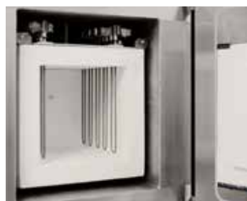
Molybdenumdisilicide heater and fiber insulation
