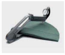
**The SG300 Substance Gauge** is a precision instrument that measures the thickness of leather. It is ergonomically designed to give perfect balance and is able to measure a greater depth of softer material than conventional units due to its unique triangular shaped frame.
