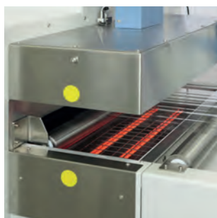
Infrared predryer for optimum heat pretreatment
