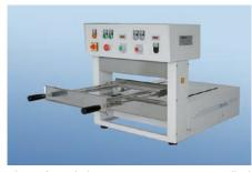
The infrared dryer type «IR-K» is installed to dry material samples which have been previously coated on a laboratory coating device type «SV».
