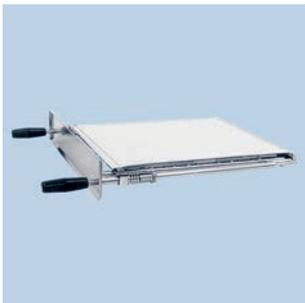
Pin frame, adjustable in length and width
