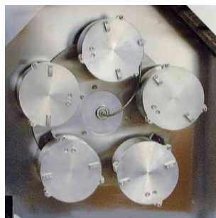
LABOMAT «BFA-24» with 5 dye beakers of 3 litres each
