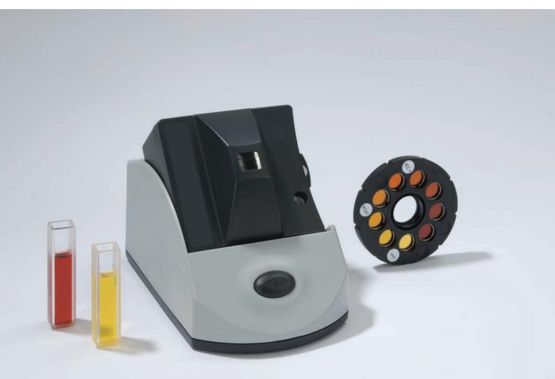
The Gardner Color Scale is a simple, visual test for measuring the color of varnishes, drying oils, resins, nitro-cellulose, lacquers, fatty acids, and similar transparent colored liquids.
