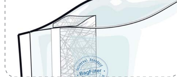
Lateral filter, ideal for fibrous sample
