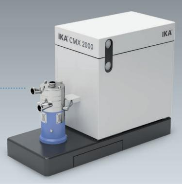
Incorporating powders into liquids, without lumps and without dust, is an important part of many processes. The CMX 2000 utilizes a specially designed rotor that creates enormous suction to draw in solids, while it pumps the liquid at the same time. The liquid can then be re-circulated until all powders are incorporated.
