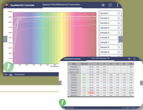
Among the many features built-in are customizable workspaces, multiple data views, and the most widely used transmission color and haze scales and indices available, including *Pt-Co/Hazen/APHA*, *Gardner Color*, *Haze %*, *Opalescence*, *Y Total Transmission*, *Saybolt*, *Absorbance*, *CIE Spectral Data*, and 3 major Pharmacopoeias: *US*, *EU*, and *Japanese*.
