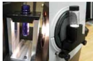
穿透用圓管夾具 / 反射用圓管夾具
