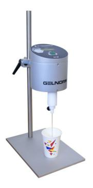
The GT-SP Slim Line Geltimer with integrated control and time measuring equipment is the compact successor model of the Geltimer TC.
