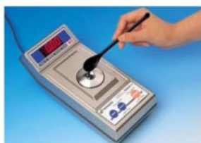
1.Drop a sample on the surface of the prism.
